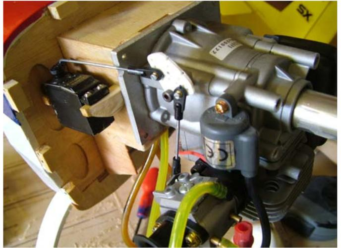
The cowl is mounted on the pre-fitted blocks with small self tapping screws.
