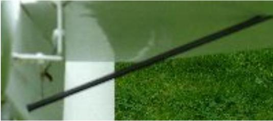
If the tailplane balsa appears to be less than fairly hard then it is worth adding some simple struts between the tailplane and fuselage on the underside. These can be made of carbon fiber tube of 5 or 6mm and epoxied into the tailplane and the fuselage sides.
