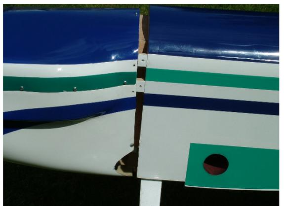
Cooling holes are cut in the cowl as shown, one below the spinner and one either side. The one to the left of the cowl is either omitted as shown or blocked to prevent too much airflow over the carb.
