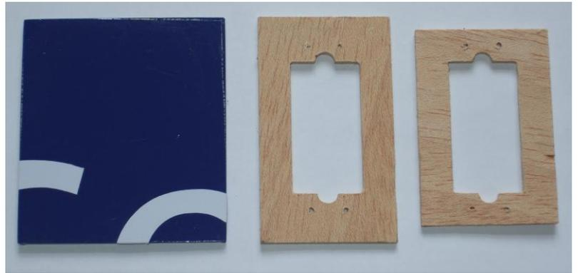
Now use the plates as a template to mark the underside of the hatch before cutting out the hatch to clear the servo. I like to cut the hatch with the servo in the middle and to clear the lugs of the servo as well so that the servo is slightly recessed.
