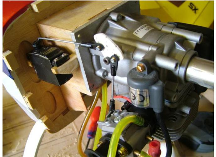
A large cooling hole should be cut in the lower rear of the cowl together with suitable air inlet holes for air to pass over the silencer with a glow motor fitted.
