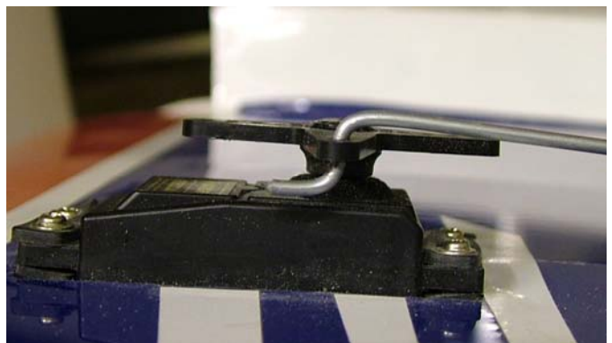
Simple joggle at servo end of 2mm pushrod.
