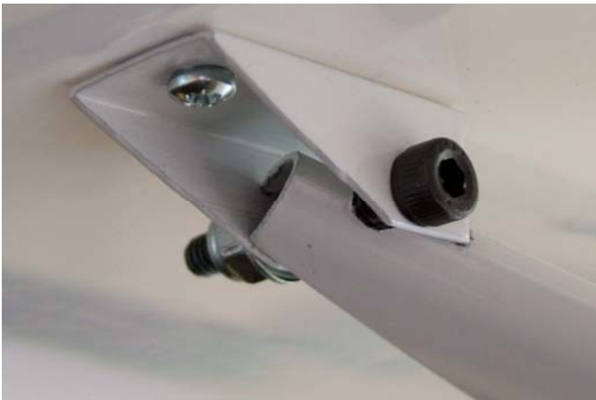
Struts fitted to wing on 92 and 111"
