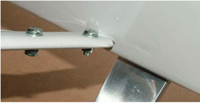
Struts fitted to fuselage on 92 and 111"
