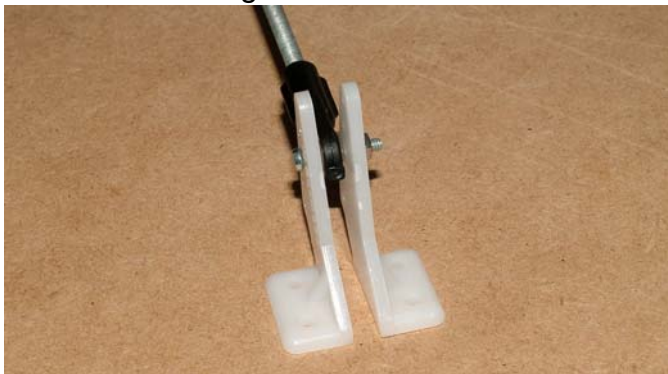
Double horns and ball links on 92 and 111"
