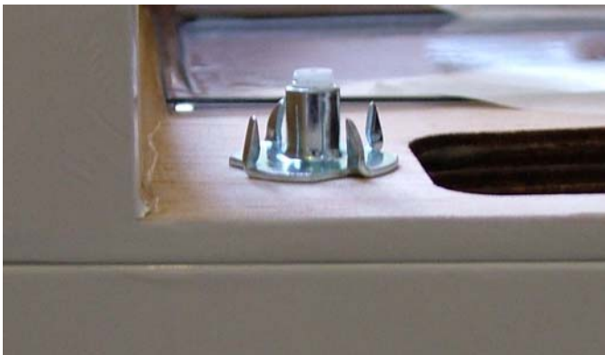
Wings secured with M5 T-nuts.
