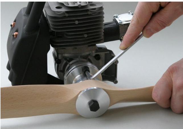
The propeller is again firmly fixed to the hub to assist in fixing the two socket head screws. Do not use Loctite, as the screws have an integrated spring washer. These screws are torqued to 10 Nm or 7 lbsft ...
