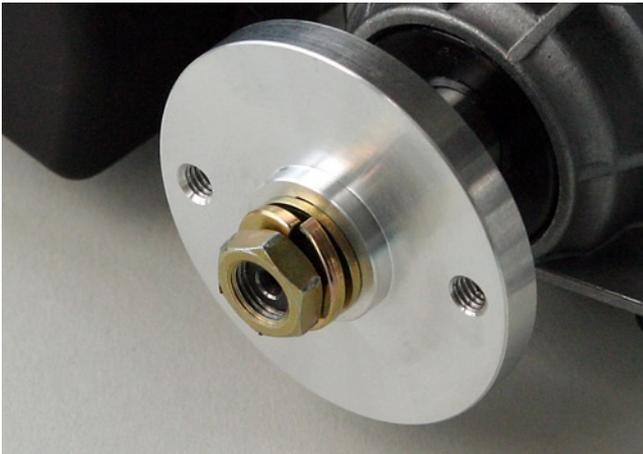
Here the adaptor has taken the place of the fly-wheel, being secured with the same nut, spring-washer and washer. Do not use Loctite as this will make dismantling unnecessarily difficult. The spring washer is totally reliable.
