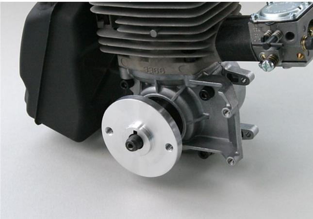
Push the propeller hub adapter onto the crankshaft taking care to see the Woodruff key is aligned with the slot. It is ideal that the adapter fits relatively tightly, the slot for the key should have no play.
