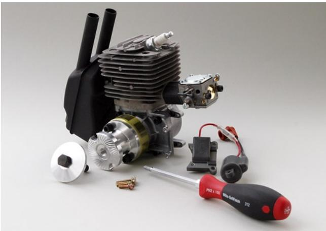
Remove the ignition and the power coil, keep the screws for fitting the sensor.
